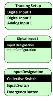
STEP 2 – Checking the existing collective switch configuration
