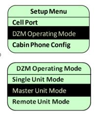
The Computer icon  $\square$  is used to indicate that a DZM is configured as a Master when using two DZMs in a Master/Remote configuration.
