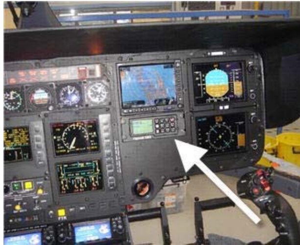
FIG: Flightcell® DZM unit mounted in Eurocopter EC135
